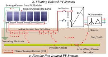
Fig. 4. Graphical Illustration of Stray Current Corrosion
