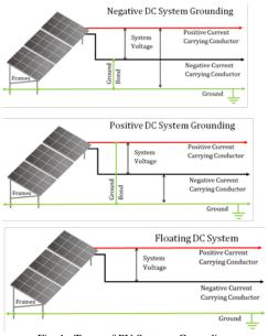
Fig. 1. Types of PV Systems Grounding
