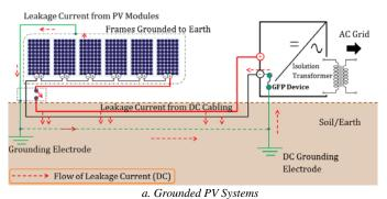
Leakage Current from PV Modules
