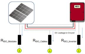
Fig. 2. Effective Insulation Resistance ( $R_{\rm ISO}$ ) of a PV System Decomposed in Constituent Elements
